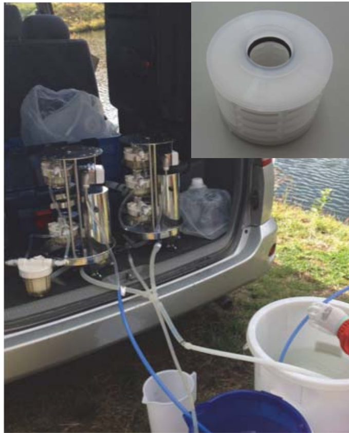
Nonwoven fabric impregnated With Prussian blue
