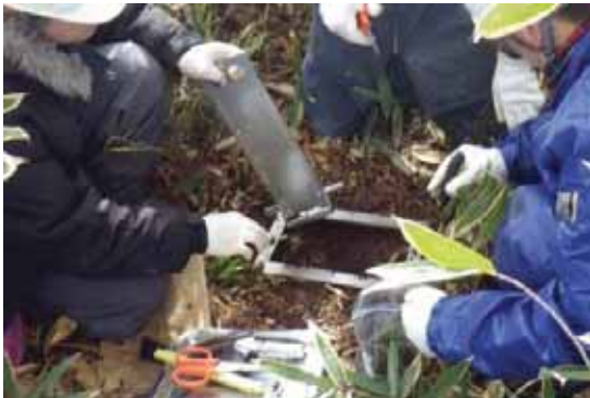
Soil sampling by scraper plate (sampling interval: 0.5 cm, 1 cm)
